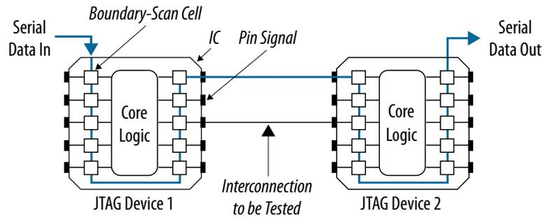
Because the JTAG interface shifts in any information to the device, leaves a low footprint, and is available on all Intel devices, it is considered a general purpose communication interface. In addition to boundary scan applications, Intel devices use the JTAG port for other applications, such as device configuration and on-chip debugging features available in the Intel Quartus Prime software.
