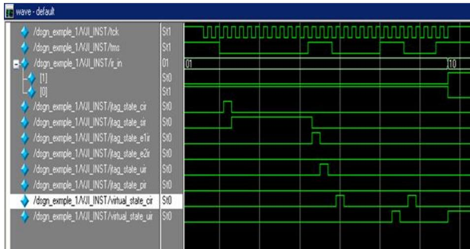
The figure below shows the inputs and outputs of the Virtual JTAG Intel FPGA IP core during a typical DR scan shift operation.
